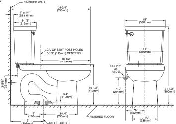
NOTES: THIS COMBINATION IS DESIGNED TO ROUGH-IN AT A MINIMUM DIMENSION OF 305MM (12") FROM FINISHED WALL TO C/L OF OUTLET. \* DIMENSION SHOWN FOR LOCATION OF SUPPLY IS SUGGESTED. SUPPLY NOT INCLUDED WITH FIXTURE AND MUST BE ORDERED SEPARATELY.
